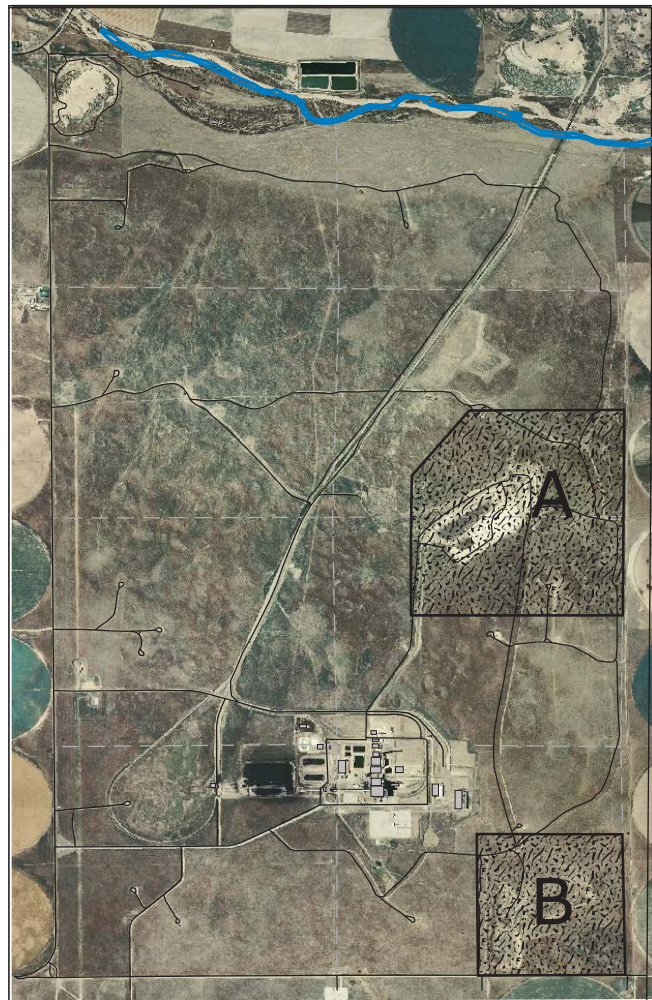
Figure 2. Digital orthophoto and map of the Sunflower Electric Site taken during 2006 and showing features and locations discussed in the text. The Sunflower Site is 2 miles wide by 3.8 mile tall and bordered on the north by the Arkansas River, on the east and west by center-pivot irrigation, and on the south by sandsage prairie. The expanded and potential landfill sites are designated sites A and B, respectively.
